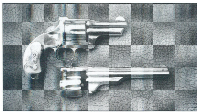
Extra barrels could be had for the Merwin-Hulbert Pocket Army, and this one also has an extra cylinder for the .44 Russian cartridge.
